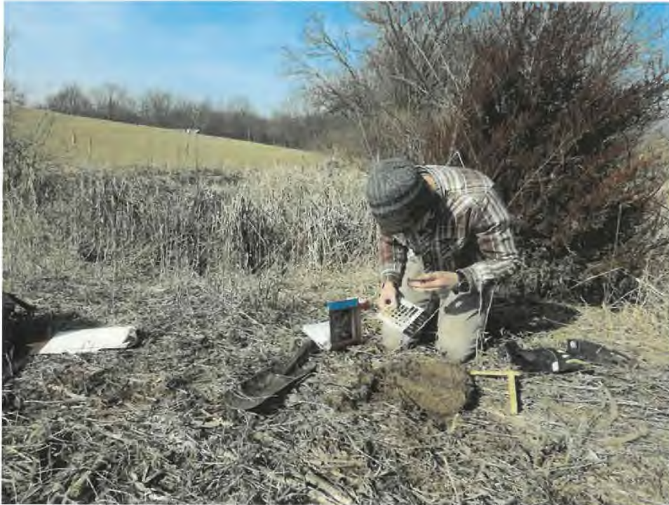
Photograph 9. MAD Scientist Associates environmental scientist, Jim Palus, describing and categorizing hydric soils in Wetland A. Photograph taken facing west.
