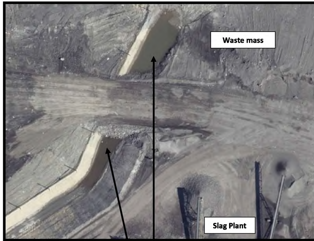
LCR Landfill Area C: Trapped stormwater soaking into the south toe of landfill creating toxic gases and leachate in violation of OAC 3745-400-11 (Q)(3) and LCR's SWPPP. Zoom.earth image
