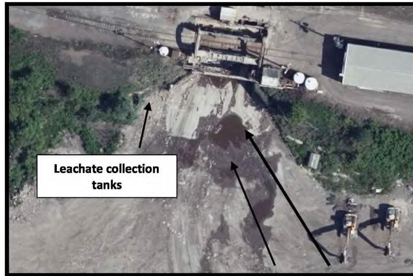
Area E: Poned waste contact water at rotary dumper does not drain to tanks but to the subsurface. Zoom.earth image
