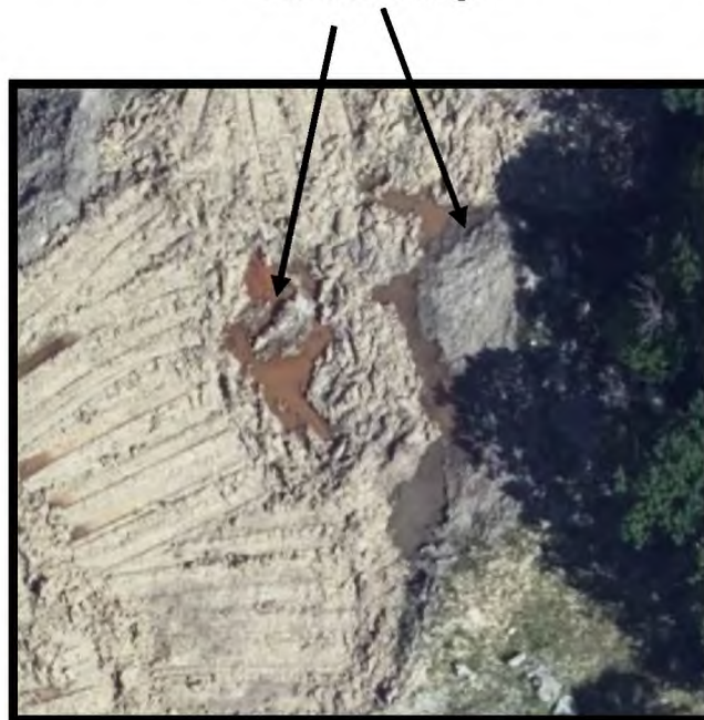
LCR Landfill Area A: Leachate/stormwater discharging east toward Palmyra Road in violation of ORC 6111, the 2017 NPDES permit, OAC 3745-400-11 (O) and (Q)(3) and LCR's SWPPP. Zoom.earth image
