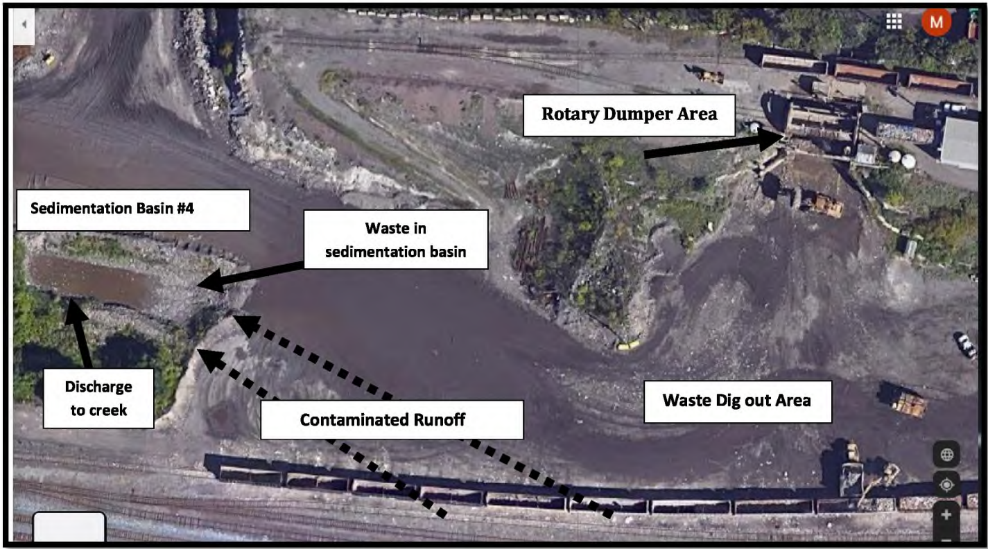
Exhibit I; Waste and leachate drain from railcars and contaminate sedimentation basin #4
