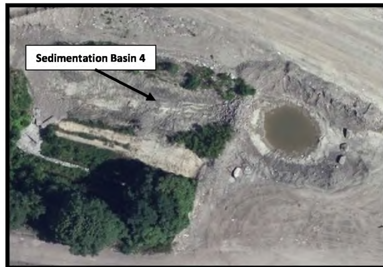
Area G: Unpermitted fore bay (to Sedimentation Pond #4 which is dry) that is collecting waste contact water from the railcar dig-out operation in violation of the 2017 NPDES permit, ORC 6111, the 2016 DFFOs and OAC 3745-400-11.
