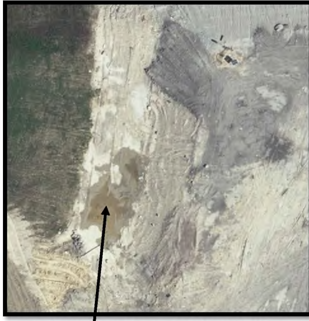
Area D: Large leachate/stormwater pond on top of landfill creating toxic gas
