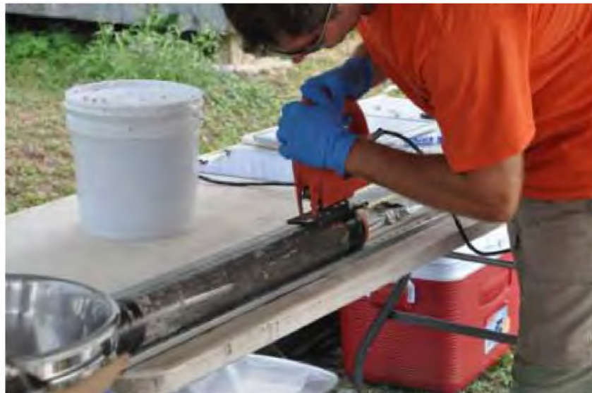
Site: Swan Creek Photograph No.: 4 Direction: North Subject: Opening polycarbonate tube from sampling location SC20-01L
