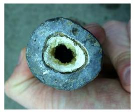
lead levels until the lead pipe is recoated. Bellaire does not add orthophosphates to prevent corrosion, they use lime instead. Below is a picture of a recently replaced LSL in Bellaire. The lime coating can be seen.
