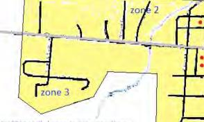
Zone 1: 1954 installed concrete main water line to copper service line to shutoff valves. Zone 2: 1988 installed ductile iron pipe to main water line to copper service line to shutoff valves. Zone 3: 2002 installed plastic main water line to plastic service line to shutoff valves. Zone 4: 2015 installed black plastic main water line to copper service line to shutoff valves North
