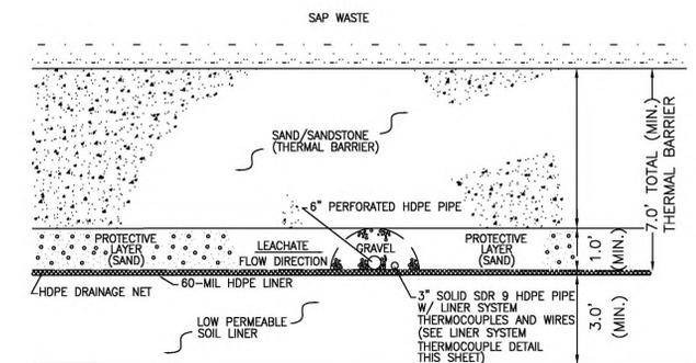
SECONDARY ALUMINUM PRODUCTION WASTE THERMAL BARRIER DETAIL
