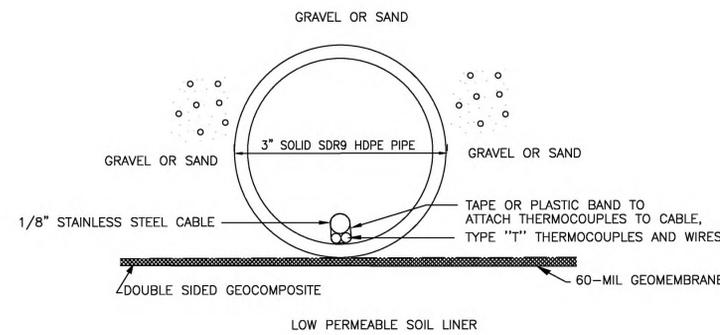
LINER SYSTEM THERMOCOUPLE
