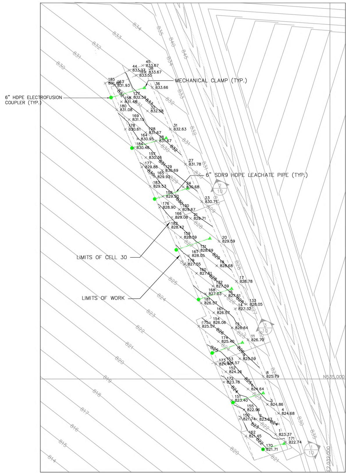
TOP OF CONSTRUCTED SOIL LINER COMPARED TO PTI TOP OF SOIL LINER
