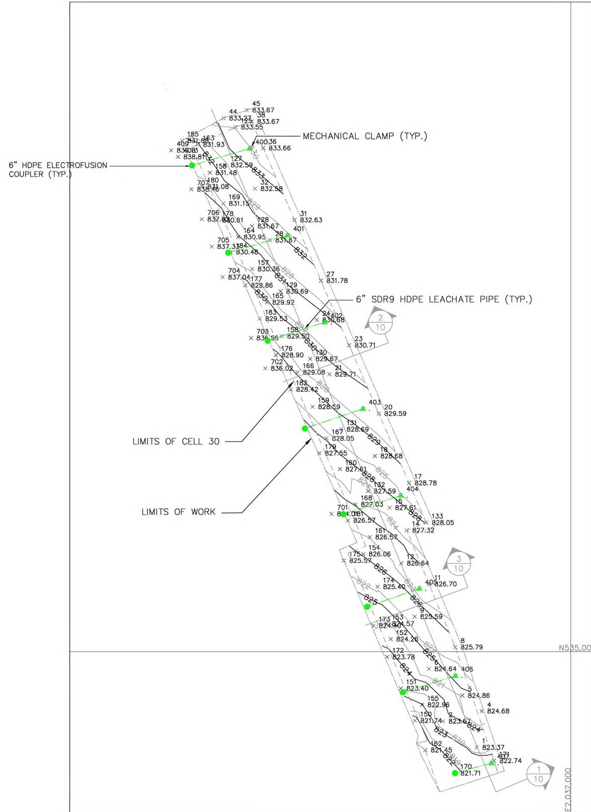
TOP OF CONSTRUCTED SOIL LINER COMPARED TO CONSTRUCTED BOTTOM OF SOIL LINER
