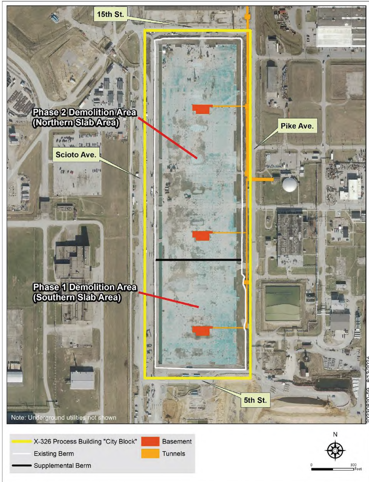
Figure 3. Location of the Remaining X-326 Process Building At- and Below-grade Structures
